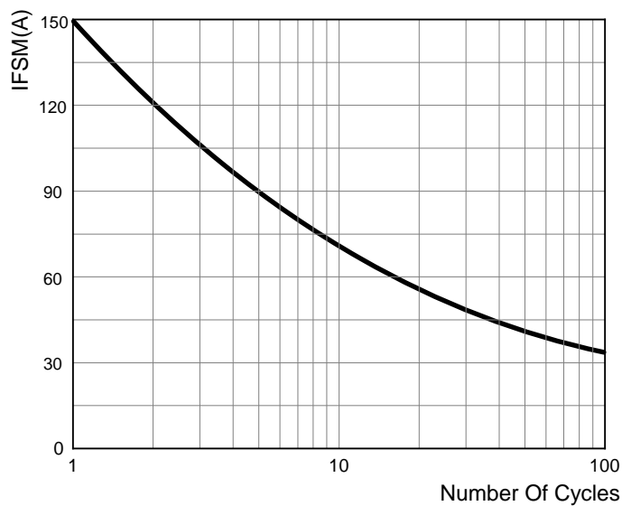
FIG 2: MAXIMUM NON-REPETITIVE FORWARD SURGE CURRENT
